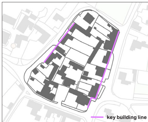
Figure 53: The block created by Main Street, Back Lane and Bell Lane features a layout somewhere between a perimeter and a more informal block. This is the highest density area of the village, and features relatively defined building lines.
