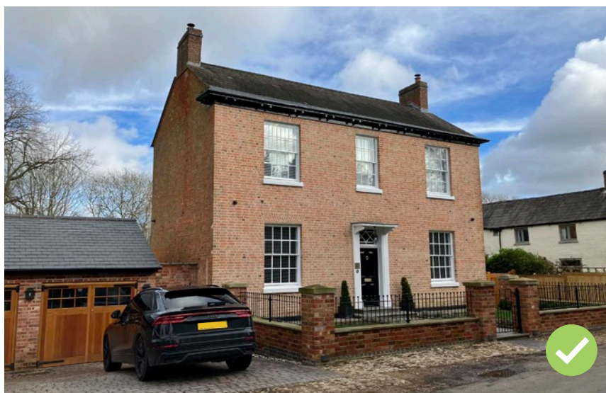
Figure 69: A good example of on-plot parking being provided to the side of a property, allowing for a small front garden to be retained. The new garage is set back behind the building line and only one storey in scale, meaning it doesn't detract from the character.
